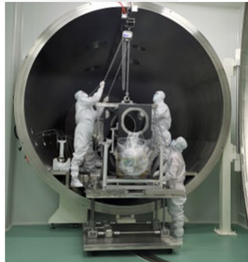
The 100XF overall schematic (up), Multi-target X-ray source (down left), EP-FXT is prepared for test in the vacuum chamber (down right)
